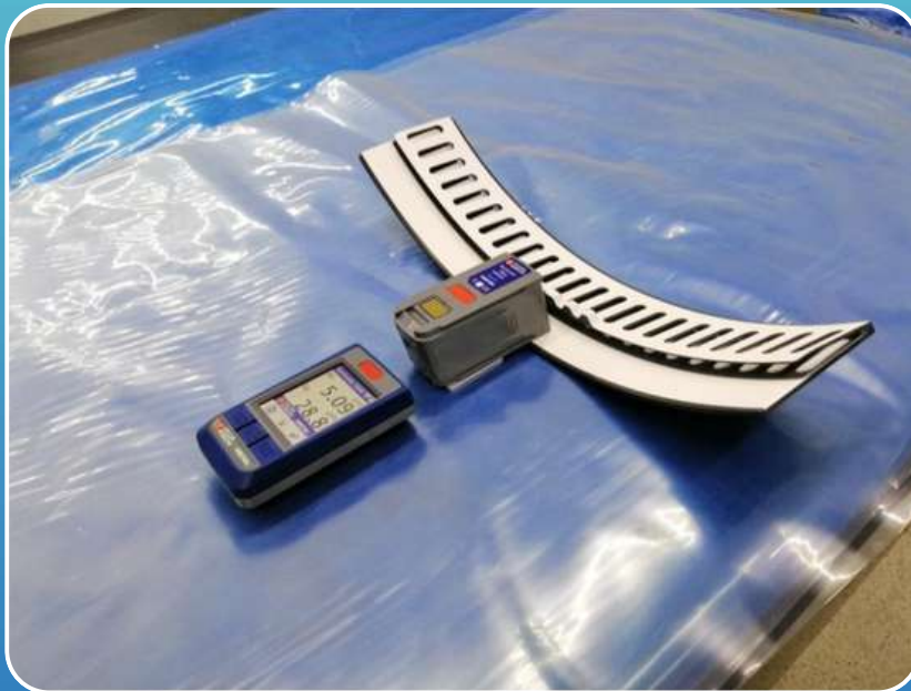
QC Coating Roughness Measurement
