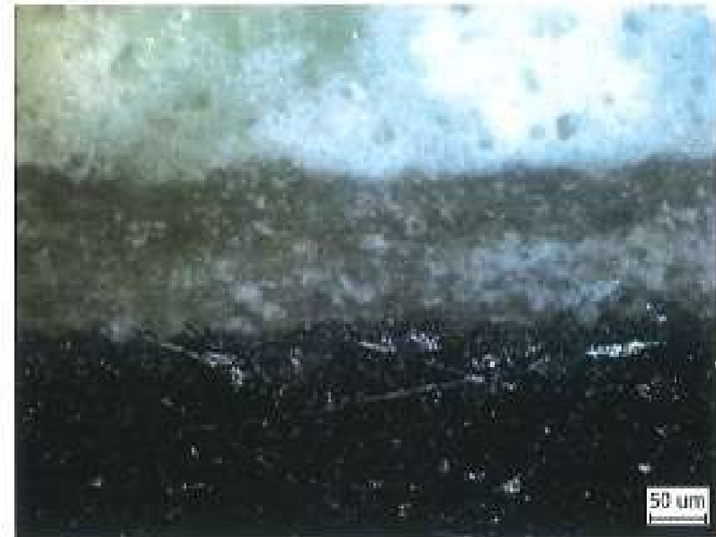
Figure 3: Typical cross-sectional view of the coating for test coupon 'PCR', as-polished, 200X
